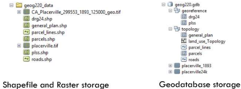
Figure 03.05. Shapefiles and raster images brought into a File Geodatabase.
